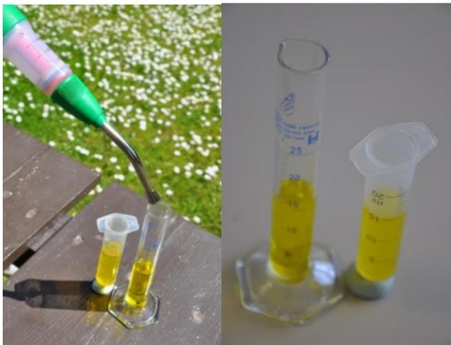
Calibration of dosing equipment can be quickly and effectively undertaken using a syringe barrel or a measuring cylinder
